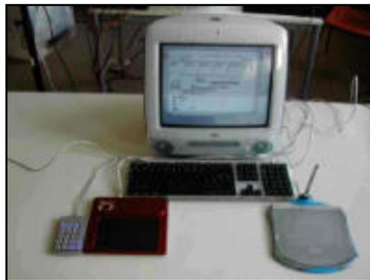
**Figure 2. The Scanned Synthesis instrument. On the right of the computer: the graphics tablet. On the left: the touch surface and the numerical keypad. The computer screen gives a visual feedback of the string motion.**
