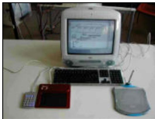
**Figure 2. The Scanned Synthesis instrument. On the right of the computer: the graphics tablet. On the left: the touch surface and the numerical keypad. The computer screen gives a visual feedback of the string motion.**
