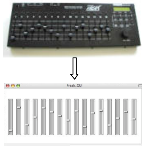
Figure 3. An example of direct control of graphical interface through a specific controller. The graphical sliders displayed on screen are permanently linked with the physical sliders of the controller.
